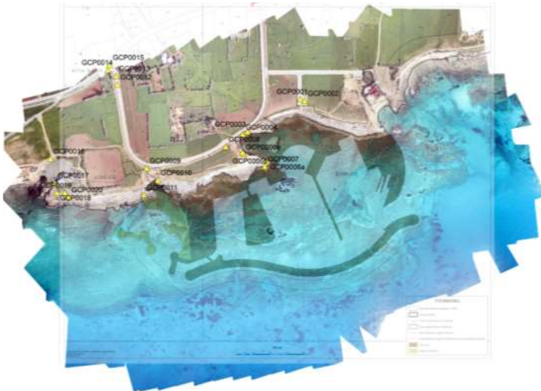
fig. 10 - Orthophotomap of Agia Napa ancient anchorage site created from initial depths, with GCPs (yellow triangles) overlaid with the marina construction plan.
