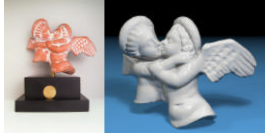
Figure 4. Eros and Psyche. Laser scanning, replica and final model, created using 15 independent point clouds.
