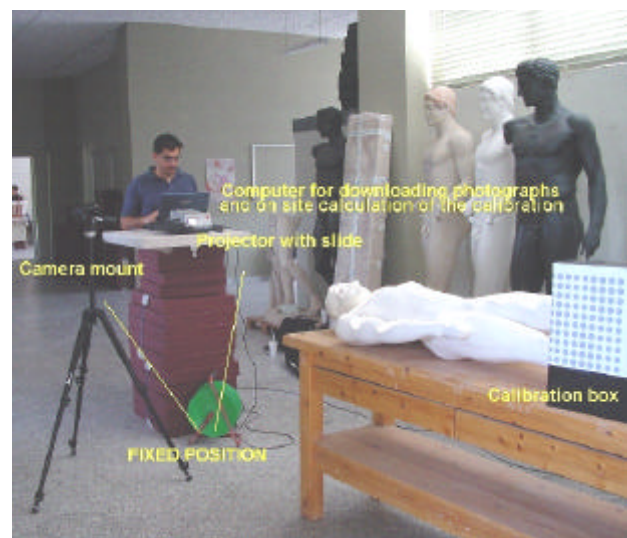
Figure 2. Set up of camera and projector during Kouros' plaster replica photography in ARF's laboratory.
