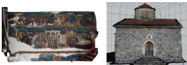
Figure 7: Results of the TLS and photogrammetric processing, orthoimage (left) and 3D rendered model (right)
