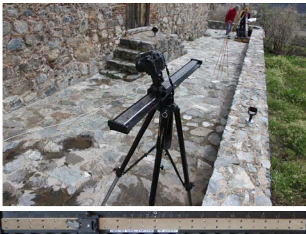
Figure 4: The typical setup of the ZScan and the slide bar
