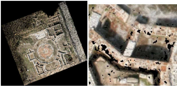
Figure 6. Orthophoto (and detail) with 0.02 m pixel size, produced using the proposed method.
