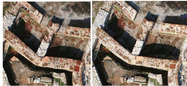
Figure 4. Orthophoto ( detail ) with 0.02 m pixel size, before and after the photo editing produced using the standard photogrammetric process.
