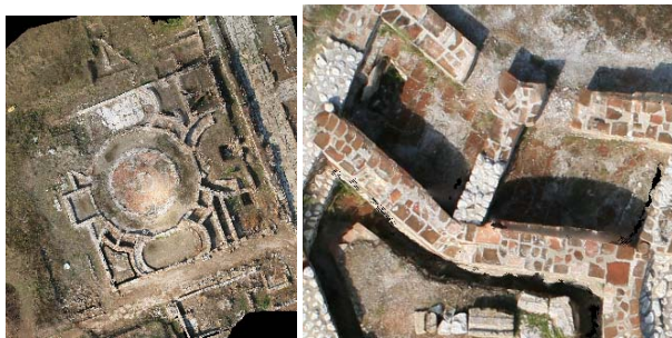
Figure 7. Orthophotograph (and detail) with 0.02 m pixel size, produced using Agisoft's Photoscan.
