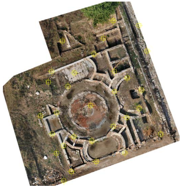
Figure 8. Points selected from land surveying, as check points to the orthophotos.
